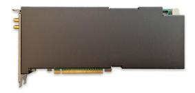
The card FB2CDG1@AGM39D-2 is equipped with 2 x QSFPDD56 for supporting 2x 400GE, as well as a wide range of other link speed combinations like 16×10/25GE or even 8x100G with the appropriate breakout modules.
