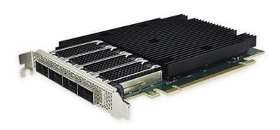
The Silicom P488CG4I81 4x100G/ 16x10G Ethernet PCI Express Gen 4.0 server adapter is based on the Intel® E810-CAM2 Ethernet controller with fully integrated four 100G Ethernet ports, is the ideal solution for implementing multiple network segments, mission-critical high-powered networking applications and environments within high performance servers.
