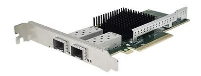
The PE425G2i81 25 Gigabit Ethernet PCI Express server adapter is based on Intel E810-XXVAM2 Ethernet controller with fully integrated 25 Gigabit Ethernet Media Access Control (MAC), and SFI Interface. In addition to managing MAC and PHY Ethernet layer functions, the controller manages PCI Express packet traffic across its transaction, link, and physical/logical layers. Using hardware acceleration, the controller offloads tasks from the host,
