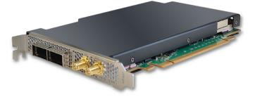
The card is based on an Intel® AgileX AGFB014, which embeds a Hard Processor System (HPS) with four 64-bit Application Processing Units (ARM Cortex-A53) along with a powerful Programmable Logic part.
