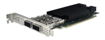
The Silicom P488CG2I81L Dual port 100G Ethernet PCIe Card Intel E810 Based is based on Intel E810-CAM1 Ethernet controller with fully integrated two 100G Ethernet Ports, enhanced programmable packet processing pipeline, virtualization (Enhanced SR-
