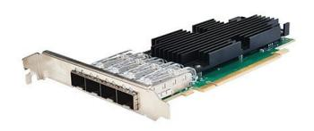
The Silicom PE425G4i81L 25 Gigabit Ethernet PCI Express server adapters is based on Intel E810-CAM1 Ethernet controller with fully integrated 25 Gigabit Ethernet Media Access Control (MAC), and SFI Interface. In addition to managing MAC and PHY Ethernet layer functions, the controller manages PCI Express packet traffic across its
