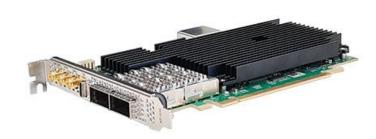
Silicom's STS3 Support 8 port of 25G/10G capabilities to synchronize host system with external clock source using 1PPS and 10MHz. The STS3 TimeSync server adapter support both 1588v2/PTP and SyncE for high clock accuracy in Master and Slave mode. STS3 design is meeting O-RAN requirements for LLS-C1, LLS-C2 and LLS-C3, modes of operations with both Boundary and Transparent clocks.
