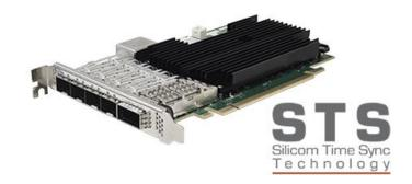
Silicom's STS2 Support 8 port of 1G/10G capabilities to synchronize host system with external clock source using 1PPS and 10MHz. The STS2 TimeSync server adapter support both 1588v2/PTP and SyncE for high clock accuracy in Master and Slave mode. STS1 design is meeting O-RAN requirements for LLS- C1, LLS-C2 and LLS-C3, modes of operations with both Boundary and Transparent clocks.
