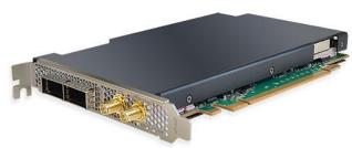
The card is based on an Intel® AgileX AGF014, which embeds a Hard Processor System (HPS) with four 64-bit Application Processing Units (ARM Cortex-A53) along with a powerful Programmable Logic part.
