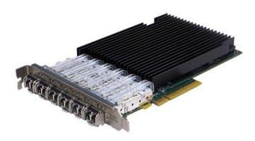
Silicom's Six Port SFP Gigabit Ethernet PCI Express Server adapter is based on Intel i350AM4 Quad port Gigabit Ethernet MAC+PHY and Intel i350AM2 Dual port Gigabit Ethernet MAC+PHY of Intel Controller.
