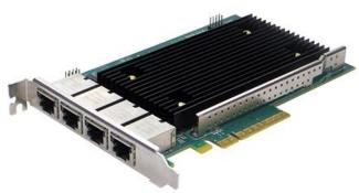
The Silicom 10 Gigabit Ethernet PCI Express server adapters are based on Intel® XL710BM1 Ethernet controller with fully integrated Gigabit Ethernet Media Access Control (MAC) and Intel® X557-AT4 10 GbE PHY. In addition to managing MAC and PHY Ethernet layer functions, the controller manages PCI Express packet
