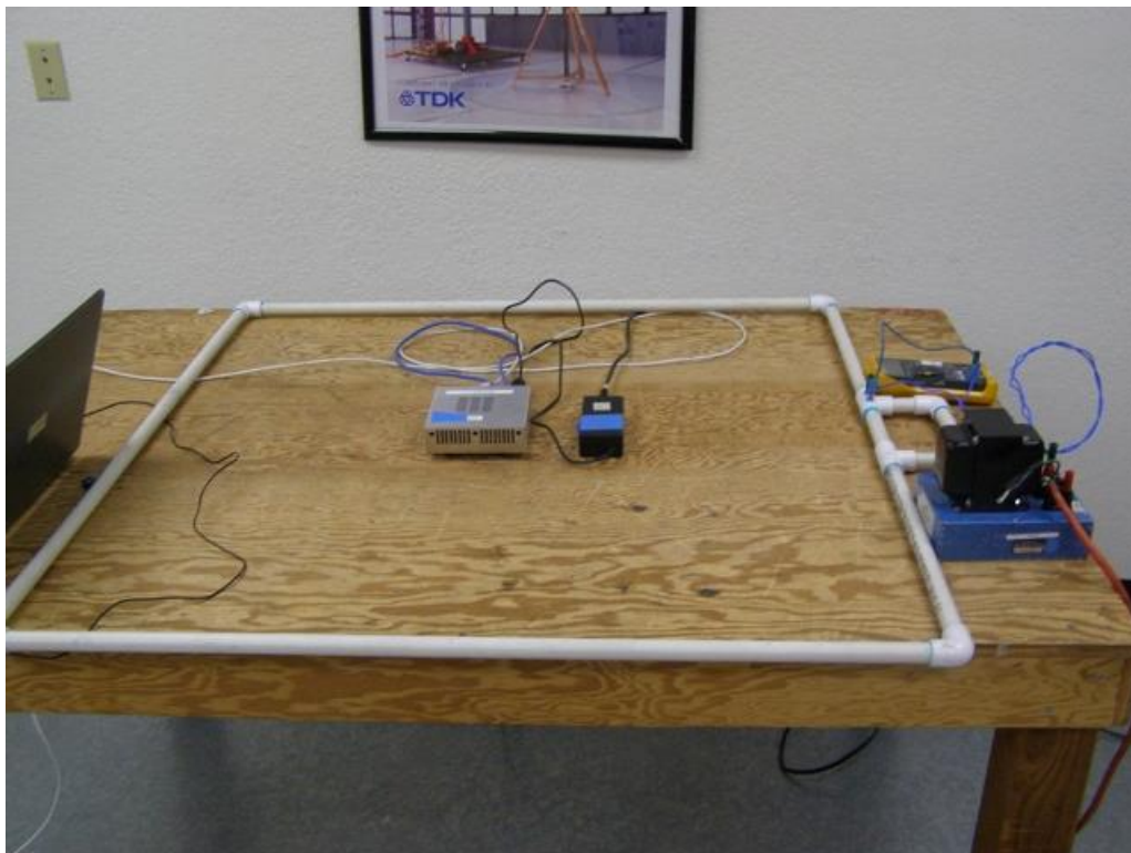
PHOTOGRAPH OF THE TEST SETUP FOR POWER FREQUENCY MAGNETIC FIELD SUSCEPTIBILITY
