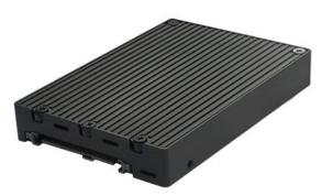
Silicom U.2 to 4 x M.2 NVMe SSD module only supports Enterprise PCIe according SFF-8639 (single x4 PCIe port), and doesn't support Dual Port Mode (PCIe Bifurcation x2x2).
