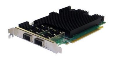
The Silicom Dual 40G / Octal 10G Gigabit Ethernet PCI Express server adapters are based on Avago PCI Express Switch and Dual Intel XL710BM1 Ethernet controllers, each with 40 Gigabit fully integrated Gigabit Ethernet Media Access Control (MAC) and XLPPI Interface. In addition to managing MAC and PHY Ethernet layer functions, the
