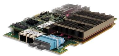
The Silicom's 6 port 100 Gigabit Ethernet add-on switch PCIe server adapter content aware packet director reduces host system process since only packets that are defined to be targeted to the host systems are routed to the host; other packets can be routed to the other port or can be dropped by the content aware hardware routing architecture.
