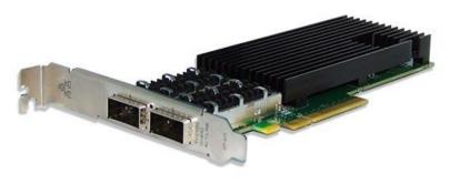
The Silicom 40 Gigabit Ethernet PCI Express server adapters are based on Intel XL710BM2 Ethernet controller with two fully integrated Gigabit Ethernet Media Access Control (MAC) and XLPPI Interface.
