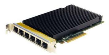
Silicom's Six Port Copper Gigabit Ethernet PCI Express Server adapter is based on Intel i350AM4 Quad port Gigabit Ethernet MAC+PHY and Intel i350AM2 Dual port Gigabit Ethernet MAC+PHY of Intel Controller. The Silicom i350 support PCI-SIG Single-Root I/O virtualization and sharing specification (SR-IOV).
