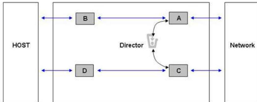
**Figure 3: Content Aware Filtering NIC Functional Block Diagram**
