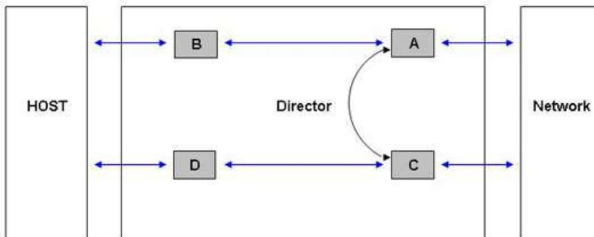
**Figure 1: Content Aware Bypass Functional Block Diagram**
