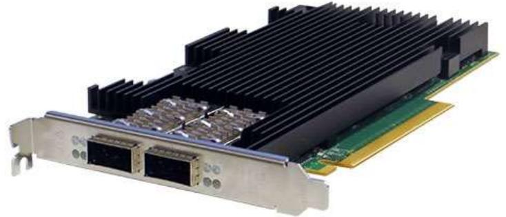
The Silicom's 100/40 Gigabit Ethernet content aware packet director reduces host system process since only packets that are defined to be targeted to the host systems are routed to the host; other packets can be routed to the other port or can be dropped by the content aware hardware routing architecture.
