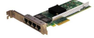
Silicom's Quad Port Copper Gigabit Ethernet PCI Express
