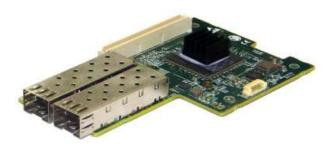
Gigabit Ethernet Media Access Control (MAC) and SFI Interface. In addition to managing MAC and PHY Ethernet layer functions, the controller manages PCI Express packet traffic across its transaction, link, and physical/logical layers. Using hardware acceleration, the controller offloads tasks from the host, such as TCP/UDP/IP checksum calculations and TCP segmentation.
