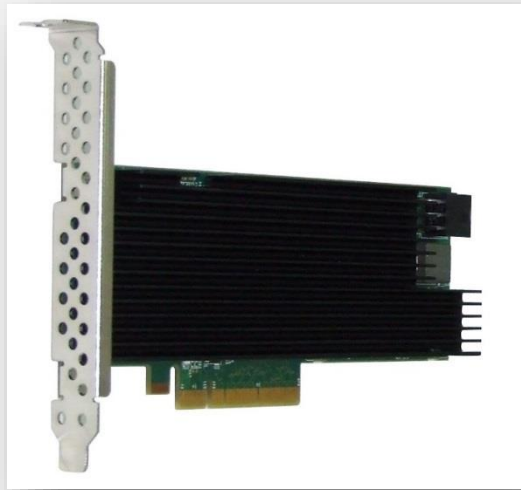
Figure 2 - Silicom PE3iSCO2 with Intel® ColettoCreek 8950 Chip Set
