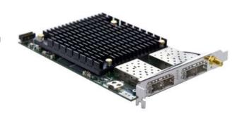
It is a high performance OEM hardware platform with four SFP+ ports, allowing for optimal flexibility in connectivity. The card allows
