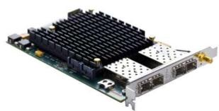
The bandwidth of PCIe Gen2 (8-lane) can provide a card-to-host memory throughput capable of supporting at least 25 Gbit/s of sustained traffic capture load.
