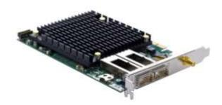
Based on powerful FPGA Hardware technology, fbC2XLG is a high performance OEM hardware platform intended for 40 Gigabit Ethernet interfacing via its dual QSFP+ slots.
