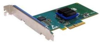
The Silicom protocol processor PCI Express adapter provides bulk cryptographic acceleration for 3DES, DES, AES and ARCFOUR symmetric encryption algorithms, for the SHA-1 and MD5 hash algorithm, and for the HMAC-SHA-1 and HMAC-MD5 keyed authentication algorithms. It provides public key acceleration for the RSA, DSA, and diffie-Helman asymmetric algorithms, as well as basic Modular Math functions.
