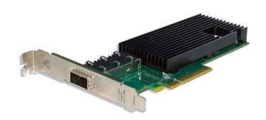
The Silicom 40 Gigabit Ethernet PCI Express server adapters are based on Intel XL710BM1 Ethernet controller with two fully integrated Gigabit Ethernet Media Access Control (MAC) and XLPPI Interface.
