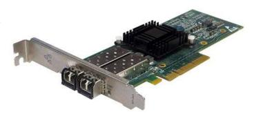
Silicom 10 GB Ethernet Cards are based on Broadcom's convergence Network Interface card (C-NIC) off load technology for iSCSI\*, FcOE\*, TOE\* and RDMA\*
