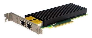
The Silicom's 10 Gigabit Ethernet PCI Express server adapters are based on Intel X540. The Intel X540 10 Gigabit Ethernet controller includes two fully integrated Ethernet Media Access Control (MAC) and two fully integrated 10GBASE-T copper PHYs.
