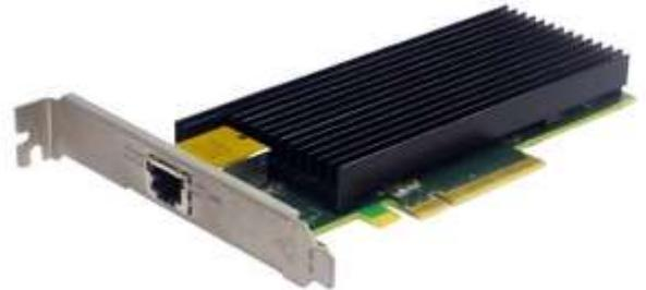
The Silicom's 10 Gigabit Ethernet PCI Express server adapters are based on Intel X540. The Intel X540 10 Gigabit Ethernet controller includes two fully integrated Ethernet Media Access Control (MAC) and two fully integrated 10GBASE-T copper PHYs .
