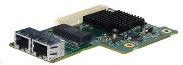
Gigabit Ethernet OCP mezzanine adapter is based on Intel I350BT2 Ethernet controller with two fully integrated Gigabit Ethernet Media Access Control (MAC) and PCI Express x4 Genereation 2.
