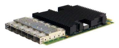
The Silicom 10 Gigabit Ethernet Express Module server adapters are based on Intel X710 Ethernet controller with four fully integrated Gigabit Ethernet Media Access Control (MAC) and SFI ports. In addition to managing MAC and PHY Ethernet layer functions, the controller manages PCI Express packet traffic across its transaction, link, and physical/logical layers. Using hardware acceleration, the controller offloads tasks from the host, such as TCP/UDP/IP checksum calculations and TCP segmentation.
