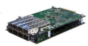
Silicom's Eight Port SFP Gigabit Ethernet ExpressModule Server adapter is designed for Servers and high-end appliances.
