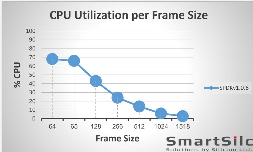
CPU power consumption emerges as yet another strength of SPDKv1.0.6, where all over fame sizes, CPU would never saturate.
