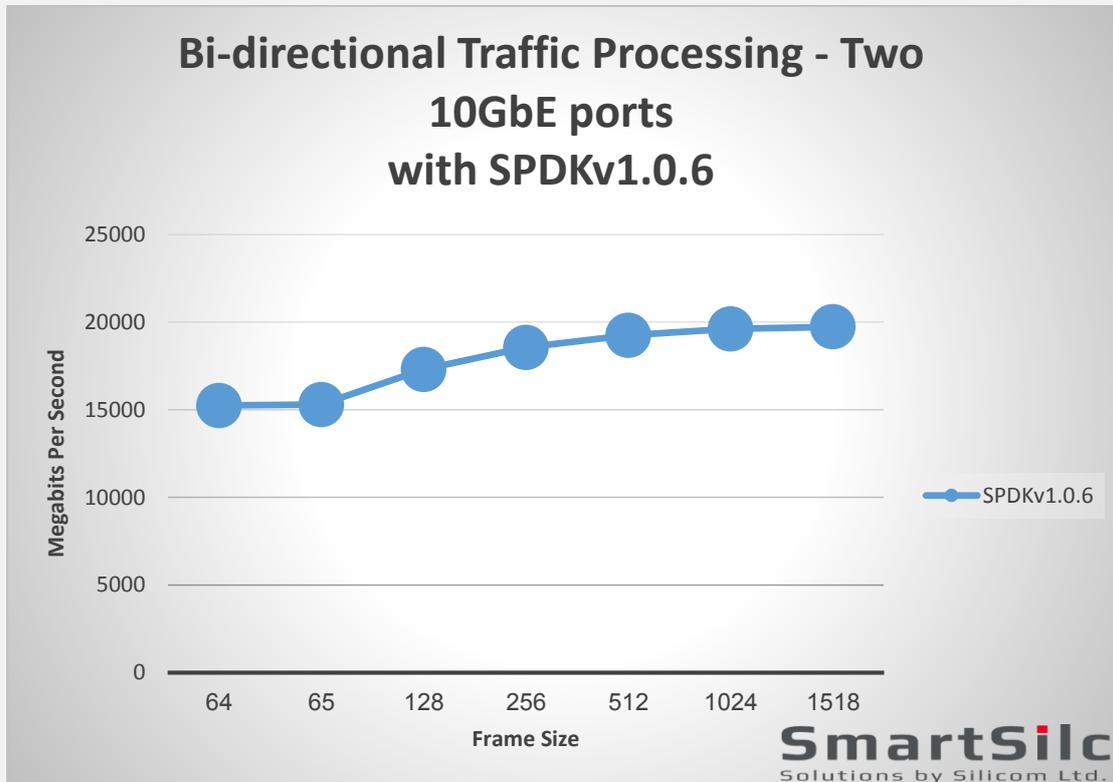
With 128 bytes long frames, SPDkV1.0.6 reaches close to the theoretical maximal bandwidth, it practically there with 256 bytes long frames. Taking into account that the rule-of-thumb average length of a data frame in the internet is ~400 long frame, we conclude that at a real life scenario, the SPDkV1.0..6 operation on a single commodity core, enabled true wire speed packet processing.
